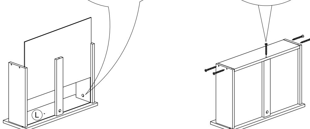
\*Assemble Drawer Side Panel-L, Drawer Side Panel-R, Drawer Crossbar & Drawer Bottom Panel to Drawer Front Panel (L) secure with Minifix (2) as shown.
