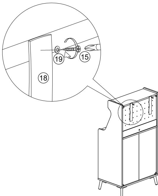
4. Add safety strap (18), washer (19) using 3.5x15mm screw (15) to back of cabinet.
