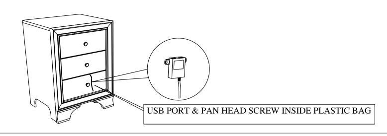
STEP 1: Assemble USB port (1) at back of night Stand (A) and fix with Screw (2) as shown.
