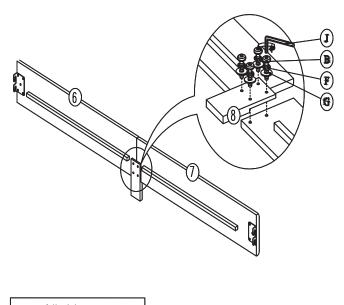
Do not fully tighten screws until assembly is complete and the bed is level
