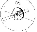
\*Attach Minifix Cap to both drawer side panels as shown.
