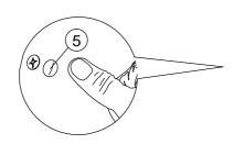
\*Attach 6 Pcs Minifix Cap (5) to panels (G) & (H) as shown.
