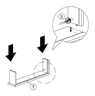
\*Assemble drawer side to drawer front (T), secure with Minifix (3) as shown.
