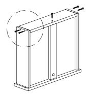
\*Assemble drawer back panel, secure with screw (8) as shown.
