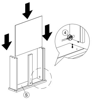
\*Assemble drawer side & drawer crossbar to drawer front (S), secure with Minifix (4) as shown.
