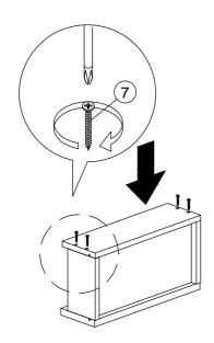
\*Assemble drawer back panel, secure with screw (7) as shown.
