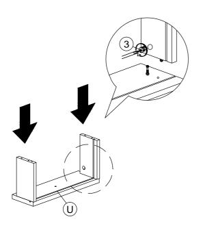
\*Assemble drawer side to drawer front (U), secure with Minifix (3) as shown.
