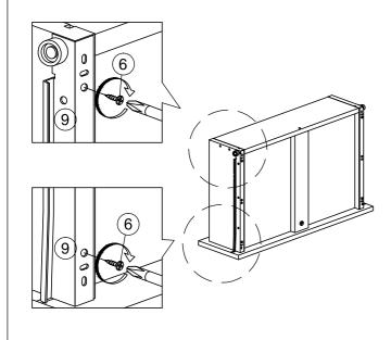
\*Assemble drawer slide (9), secure with screw (6) as shown.
