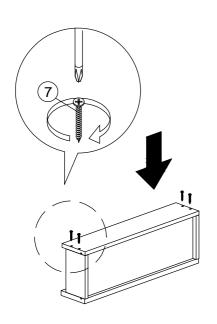
\*Assemble drawer back panel, secure with screw (7) as shown.
