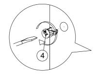
Assemble panels (B) & (E) secure with Minifix (4) as shown.
