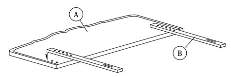
Align pre-drilled support stand holes over the pre-drilled headboard holes according to your desired headboard height
