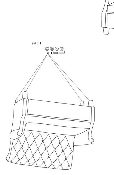
Do not tighten screws until completely assembled.
