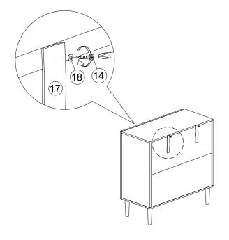
4. Add safety strap (17), washer (18) using 3.5x15mm screw (14) to back of cabinet.
