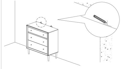
1.First mark the wall with pencil as in diagram.
