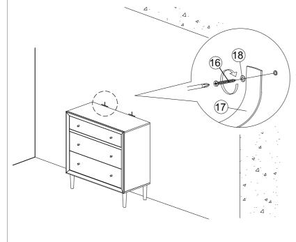
5. Finally, attach safety strap (17) and washer (18) using 4x30mm screw (16) to the wall.
