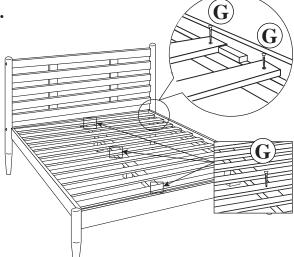
Lay the slats (P7) between the side rail (P3) using hardware:
