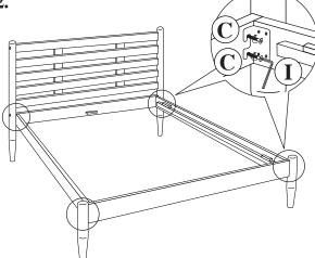
Attach the side rail (P3) to the headboard centre support (P8) and footboard (P4) using hardware:
