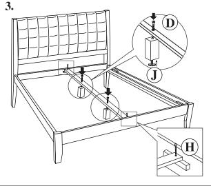
Fix the adjuster (J) to the support leg (P6) using hardware:
