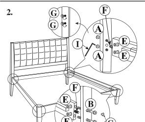
Attach the side rail (P3) to the headboard using hardware:
