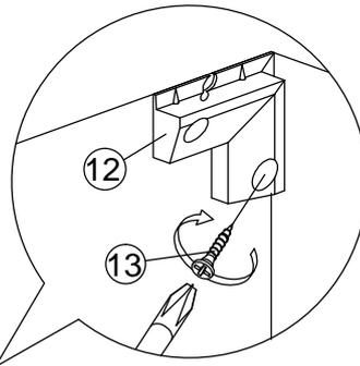
*\*Assemble Top Panel (A) with Panel (E) secure with Minifix as shown.*
