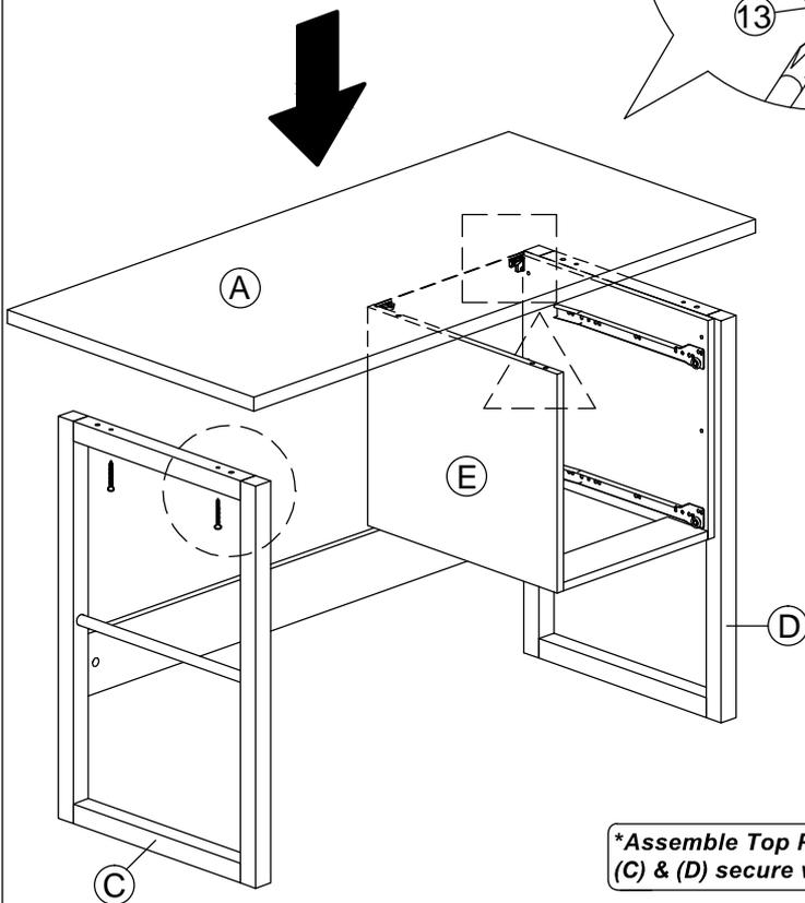
*\*Assemble Top Panel (A) with Frame (C) & (D) secure with screw as shown.*
