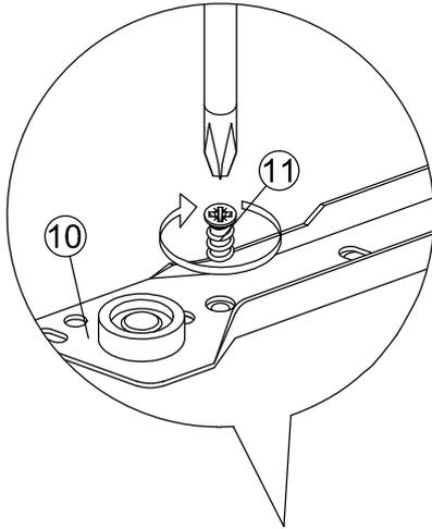
*\*Install Drawer Slide to panels (E) & (F) with screw as shown.*
