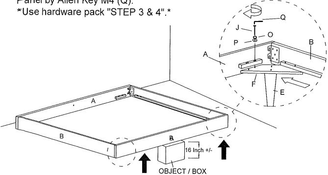
Level up the Headboard Panel (A) by putting on object/box to fix the Bed Leg (E) with the Bed Leg Support (F). Insert JCBC M6 X 50mm (J) Flat Washer M6 (P) Spring Washer M6 (O) to Headboard panel (A) connection Bed Leg Panel by Allen Key M4 (Q).
