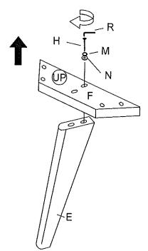
2 Insert JCBB M8 X 25mm (I) Flat Washer M8 (N) Spring Washer M8 (M) to Side Rail (B) connection Hb/Fb panel (A) by Allen Key M5 (R).
