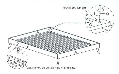
8 Insert JCBC M6 X 50mm (J) to Bed slat (G) connection Center Support (C) by Allen Key M4 (Q).
