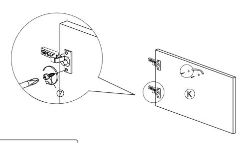
\*Install 2 pcs Hinges with TP 10#x1/2" screw as shown.
