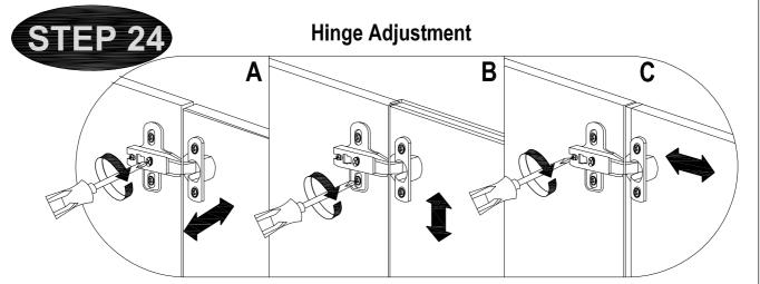
A.Lateral adjustment by screw adjusting
