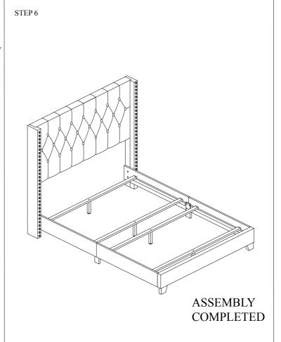
NOTE : AFTER A FEW DAYS OF ASSEMBLY , IT WILL HAVE ACCLIMATIZED TO THE ENVIRONMENT. PLEASE TIGHTEN ALL HARDWARE. CHECK TIGHTNESS OF ALL SCREWS EVERY 6-8 WEEKS.
