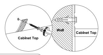
NOTE: Wall fixings are not supplied with this product as different wall materials require different types of fixing devices (such as Rawl plugs on brick work). You must use fixing devices suitable for the type of wall you intend to mount this product to.Please ensure that the head of any screw used has a diameter greater that the diameter of the mounting hole on the bracket and that the fixing is safe and secure before use.
